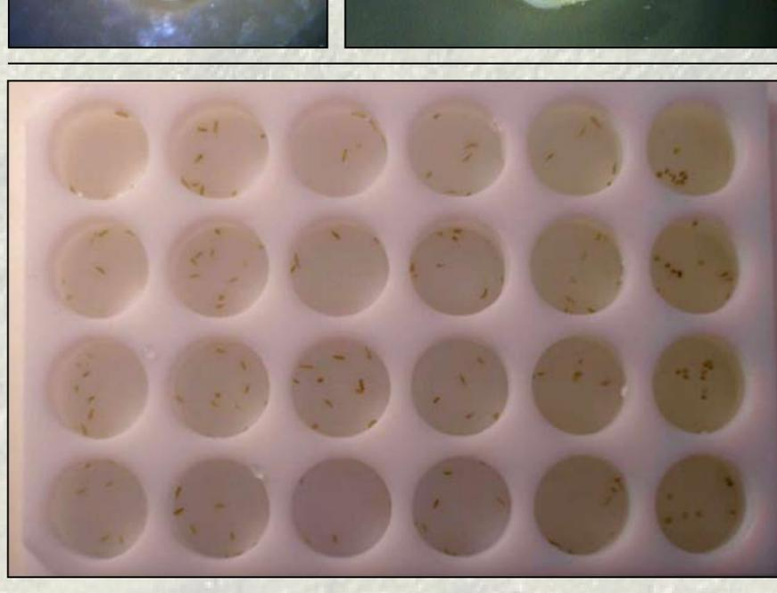
**ABOVE:** FIG.5 - Coral planula can be exposed to a pollutant using a Teflon 24-well microplate. Ten planula per well, and 4 wells per treatment. A control and five concentrations of a pollutant can be tested using a single Teflon microplate.
