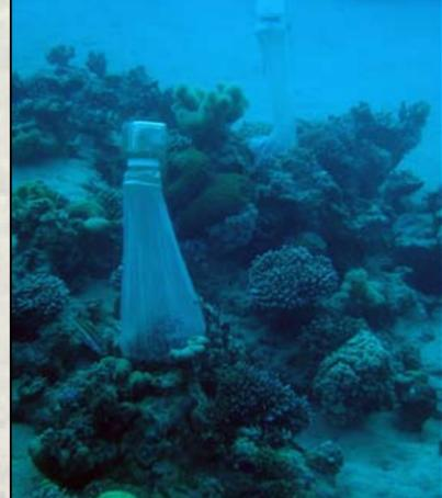
**LEFT:** FIG.3 - An air bubble in the planula trap allows the trap housing to float above the coral colony. Planulae are positively buoyant, so they will float and collect into the trap housing.
