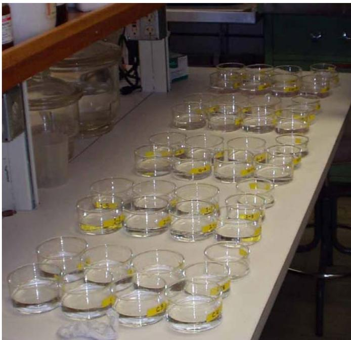
**Figure 2.1** - Pyrex dishes can be used as dosing chambers. In this picture, there are five treatments with nine replicates; each chamber is a single replicate. Unjoined chambers should be randomly configured on the laboratory bench after the xenobiotic and the larvae have been added to the chambers.
